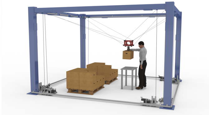
Fig. 1: Human-robot collaborative setup in which a human operator is loading a payload onto a CDPR
